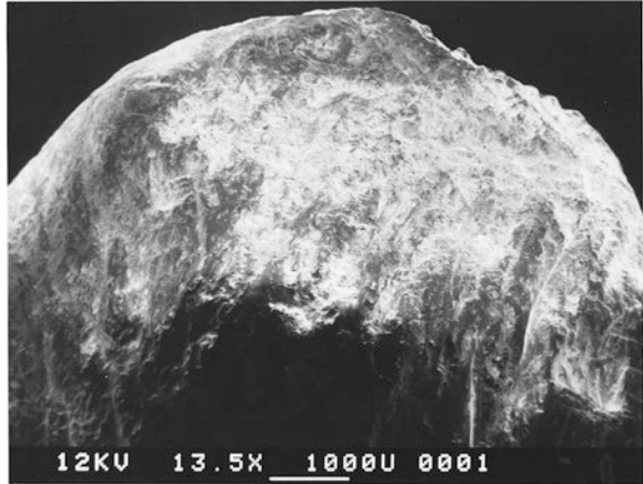
Fig. 14.17 SEM micrograph of jagged surface and striations on deer antler beam, produced by its use as a soft-hammer percussor for stone artifact production by Sandra L. Olsen (1989:132, Fig. 7). Scale: bar is 1000 microns. Compare with Fig. 13.13 for natural antler modification image. (Used with permission of S. L. Olsen and Elsevier)
